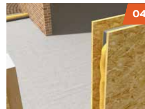
Expanding urethane sealant is used between all panel joints for superior airtightness.
