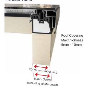
Fixings for attaching kerb to deck are not supplied.
